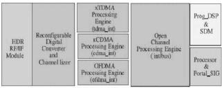
Multi-standard BTS engine for the 4G OWA platform
