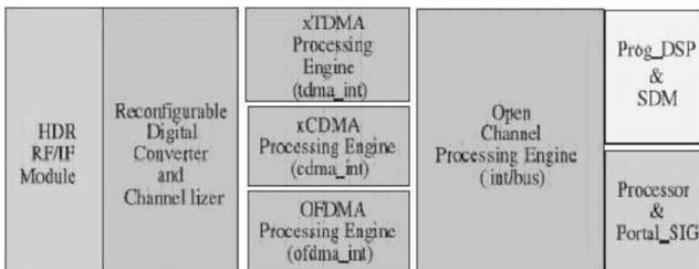
Multi-standard BTS engine for the 4G OWA platform
